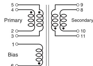
Primary windings and secondary windings to be connected in parallel on PC board.
